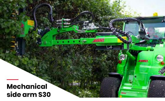
The mechanical side arm with the S30 quick attach system can be fitted with lighter (max. 200 kg) attachments like the S30 cutting bar and the S30 multi function drive unit with HD brushes. It is equipped with a mechanical, manually extendable straight telescopic arm and a hydraulic jib arm which tilts the attachment up and down. Telescoping to the side is max. 1000 mm and jib arm movement is max 45° down and 90° up from horizontal position.
