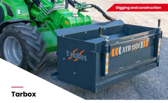
An economic attachment for placing Asphalt, Tar or any Screed materials. Ideal for pathways and areas that a placer machine cannot gain access. The AVANT Tarbox is available in 1500 mm width with 200 mm offset to both sides. A width reducing plate allows narrow trenches or strips to be filled. Material depth control is via screw control. The easy to operate TarBox will increase productivity on any job.
