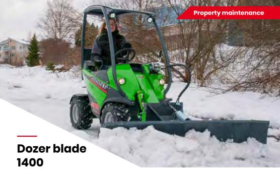
Equipped with hydraulic blade turning, Avant dozer blade is the ideal tool for snow removal, earthmoving and similar jobs where the materials must be dozed away quickly.
