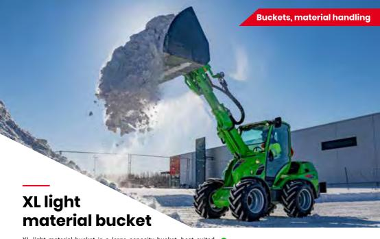
XL light material bucket is a large capacity bucket, best suited to Avant 600, 700 and 800 series. It is intended for loading and transporting of light materials like wood chips, mulch, snow etc. There are no reinforcement plates inside the bucket which would interfere when loading and emptying, and the sides open forward in a slight angle, which guarantees easy and complete emptying of all kinds of materials and in difficult conditions also.
