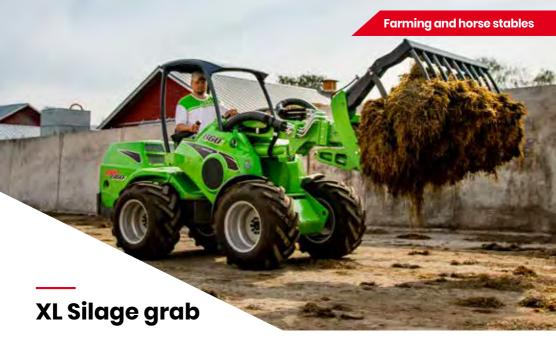
The larger silage grab series is intended for Avant 500, 600, 700 and 800 series loaders, with three different widths to match machines perfectly. The new series can carry up to 30 % more silage without losing visibility on the feeding table. Open grab construction on the top offers better visibility when the grab is open. Strong heavy duty construction with two cylinders. Forged bolt-on tines also on the top grab.
