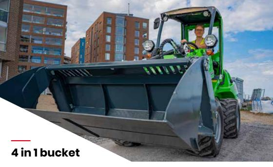
Efficient multi purpose bucket - can be used as a normal bucket as well as a dozer blade, leveler or a grab. The front part of the bucket opens with 2 hydraulic cylinders, located on the back side of the bucket, which enables dozing, levelling and picking of stones, tree stumps etc. Another benefit of the opening bottom is that the bucket can be emptied at a higher level by opening the bottom instead of tipping the bucket edge down.
