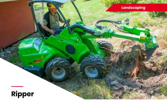
The ripper is an inexpensive and practically irreplaceable tool in On An inexpensive tool for removing ground works. With the ripper it is easy and effortless to remove roots as well as rocks even from hard packed ground. The replaceable hard metal teeth guarantee a long lifespan for the attachment.
