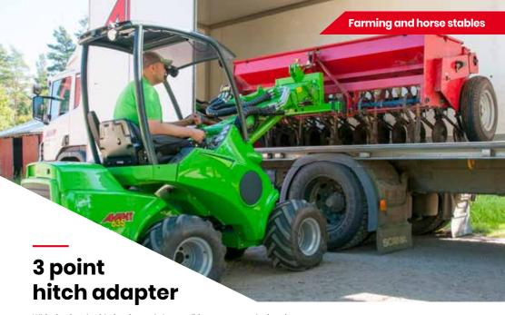
With the 3 point hitch adpater it is possible to move agricultural attachments with Avant, for instance for storage, cleaning etc. This can be practical especially when space is limited and handling with tractor is difficult. Also the trailer ball hitches can be mounted on the 3 point hitch adapter.
