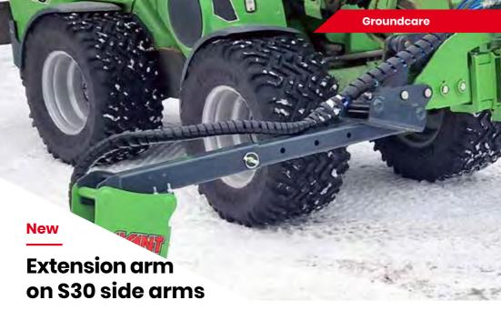
The optional extension arm with manually extendable telescope can be mounted both on the hydraulic and on the mechanical S30 side arm. It gives extra outreach and working height with certain S30 attachments like the branch cutter and cutting bars. The extension arm can be locked with a bolt in four different outreach positions: without telescoping 550 mm, then 620, 780 or 950 mm. The arm also comes with the hydraulic hose extension kit A412129 (3 pcs 800 mm long hoses) for the attachment.
