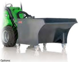
A418506 Castor wheels, 4 pcs (will increase bucket height by 165 mm) A420800 Castor wheels, pneumatic tires, 4 pcs will increase bucket height by 235 mm) A420537 Supports, 4 pcs
