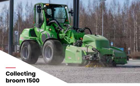
The collecting broom 1500 is mainly intended for professional property maintenance companies, cities and municipalities. The broom has a heavy duty construction, floating brush axle, automatic brush wear compensation and a specially designed water spraying system for dust binding.
