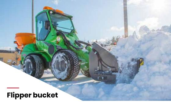
Flipper bucket is designed for clearing snow in large areas or in areas where snow must be moved long distances. Thanks to the two hydraulically operated side wings the bucket is exteremely versatile in snow clearing and can be operated in smaller areas as well without problems.
