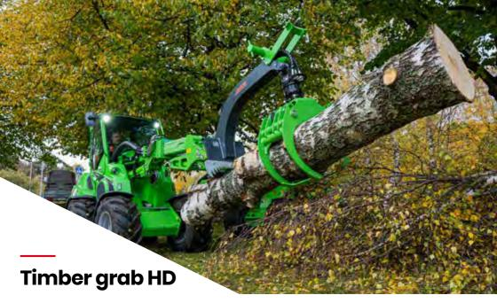
The heavy duty timber grab is equipped with a stronger boom and hydraulic rotator and larger grapple. It is intended especially for Avant 700 and 800 series. The arborist kit which mounts on the boom is also standard feature. When cutting a tree you can push the tree down with it if necessary, instead of pushing by hand. It is also possible to attach a rope on the bracket on the kit, which enables towing the logs by pulling them with the loader.
