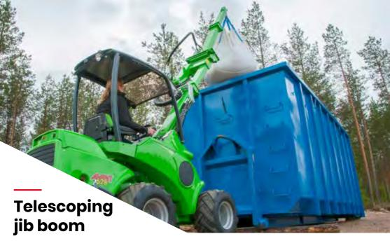
The hydraulically telescoping jib boom is a very efficient and versatile tool in all lifting jobs on the work site. The steplessly extending and retracting boom allows lifting to places that would otherwise be very hard to reach. Compact design with telescoping cylinder inside the boom makes work safe and easy.
