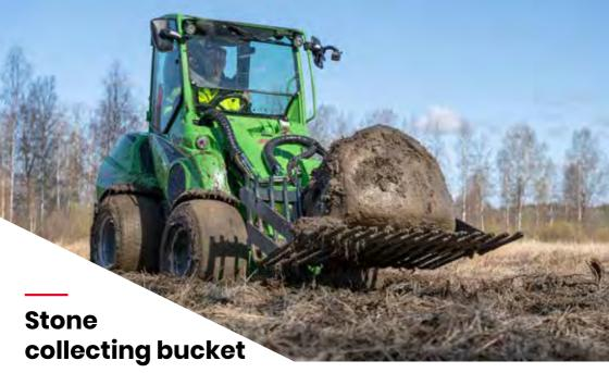
The stone collecting bucket - also known as riddle bucket - is intended mainly for collecting stones from the fields after the field has been harrowed. With an Avant it is easy and fast to collect stones from nearby fields.
