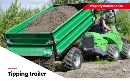
Avant tipping trailer is available in two models: with carrying capacity of 1200 kg or 1800 kg. Both are equipped with hydraulic tipping. All sides can be removed if necessary. Extra side set is available as an option for the smaller model, on the bigger model it is standard.
