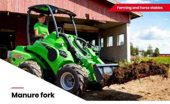
Avant manure fork is a very useful attachment, designed for detaching and handling of manure and similar materials. The strong tines, made of high tensile forged steel, penetrate also into compacted manure and can carry a heavy load.
