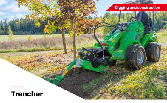
With Avant and trencher you can easily dig narrow trenches without damaging the ground on the digging area. The trencher does a clean trench which can easily be filled with a bucket or a dozer blade. Planetary drive with hydraulic motor guarantee powerful and trouble free operation.
