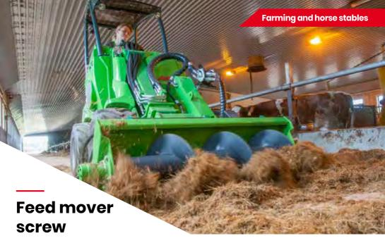
Efficient way of moving uneaten feed back in front of the cattle. When moving, the screw mixes the feed and the fresh feed remains
