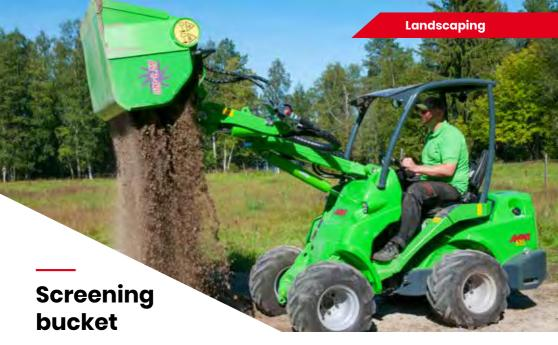
The Avant screening bucket is a fast and efficient compact system for screening and blending soils, aggregates and compost. The durable and flexible star-shaped plastic Poly Star rollers screen without shredding the vegetation or crushing the aggregates into the finished screened product.
