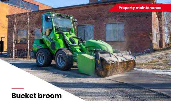
Bucket broom collects the waste in a large bucket shaped box. The broom gives best sweeping result when reversing, but it also works when driving forward. Forward sweeping is especially recommended when the waste is larger in dimensions, for instance construction waste, beverage cups, tree leaves etc.
