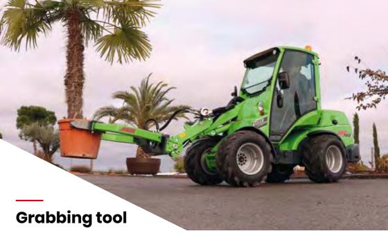
Grabbing tool is mainly intended for lifting and handling of round objects. It is especially suited for lifting of barrels and plant and tree pots. Grabbing force can be adjusted, which means all kinds of objects can be handled without damaging them.
