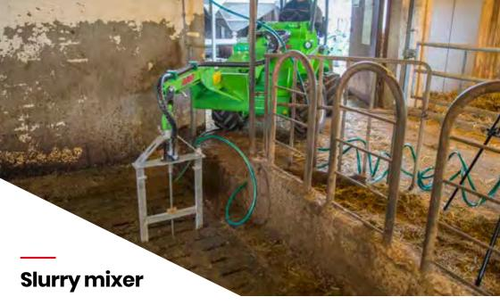
Slurry mixer is a special attachment for cattle farms: in cattle buildings with slatted floors, where the animal waste falls through the slats directly to the storage tank below the floor. The slurry that forms in the tank needs to be mixed from time to time in order that it stays liquid and moves towards the bigger slurry container which is usually located outside the building.
