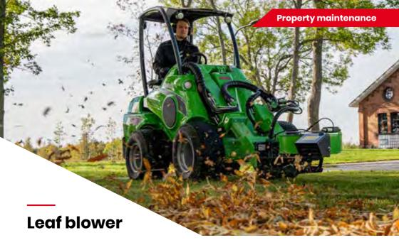
With the leaf blower you can easily and quickly move away large amount of leaves from lawns, yards, sidewalks etc. The hydraulic motor powered blower is very efficient and the big tiltable nozzle blows the leaves away from a large area.
