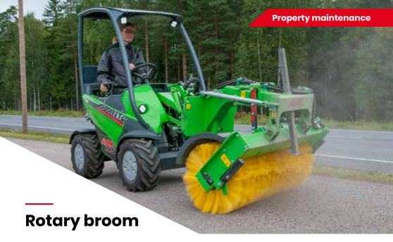
Avant rotary broom is an efficient and easy to use attachment for various cleaning jobs. Three working widths available, 1100, 1500 and 2000 mm. The 1500 and 2000 mm brooms are equipped as standard with turning which is powered by electric actuator motor. This means turning of the broom is easily and comfortably operated with a switch from the driver's seat.
