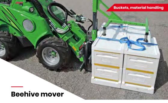
Avant beehive mover is intended basically for loading and transporting of beehive boxes, but it can handle other objects like cardboard boxes as well. The mover can carry as many as 12 beehives at a time. It consists of a mast, a pallet fork that is mounted on the lower end of the mast, and a hydraulic grapple at the upper end of the mast which presses the boxes against the pallet fork. The grapple is equipped with rubber pads which hold the beehives firmly but gently.
