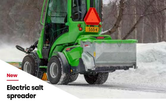
The electric powered salt spreader features a traditional bucket design and can be mounted on the front or rear of the loader. To avoid salt dust corrosion on the loader, rear mounting is recommended. The spreader is made of hot-dipped galvanized Robust design, made of hot-dipped steel and the shaft of stainless steel.
