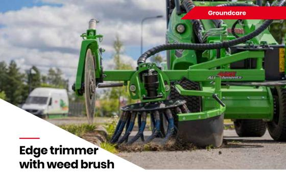
The edge trimmer equipped with a weed brush allows lawn edge cutting and sweeping at the same time. It is intended for cleaning the edge between kerb stones and lawn, and it can also be used for trimming the edge between the lawn and paving, asphalt, concrete slab. etc.
