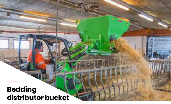
The bedding distributor bucket is intended for distribution of different types of beddings in cowhouses, poultry farms etc. The bucket is equipped with a 300 mm wide belt, which allows distribution of chopped straw, sawdust, peat, bark, wood shavings, sand and lime. Belt speed is steplessly adjustable.
