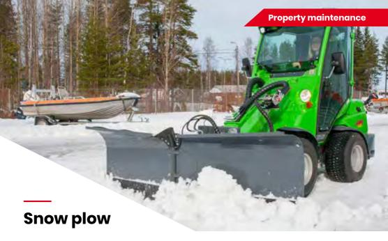
Avant snow plow is a versatile attachment for snow removal. It consists of two independently hydraulically adjustable blades. Angle of the blades is be adjusted with a switch from the driver's seat. Both blades have a spring release mechanism in the lower part of the blade to prevent any sudden stop should the blade hit an obstacle. The floating mechanism on the mounting bracket guarantees that the blade follows ground as well as possible.
