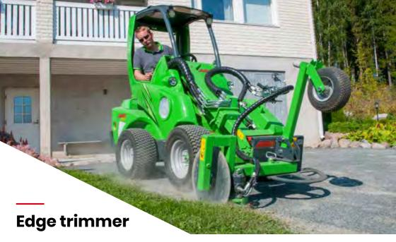
Avant edge trimmer is the perfect attachment for trimming Cuts the lawn edge accurately, the edges of lawns, hedges, flower beds etc. It consists of a hydraulically operated trimmer mounted next to a cutting disc.
