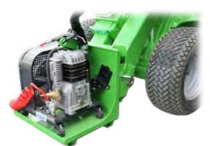
air flow / pressure max. 400 I / 8 bar Oil flow range 10-21 l/m (Auxiliary hydraulics) Product no A35409
