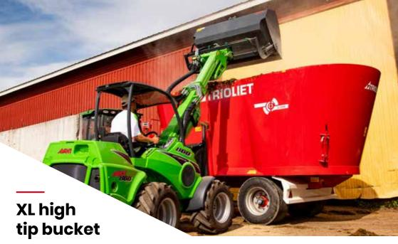
The XL high tip bucket has more loading volume - very useful when loading light materials. The bucket is an ideal tool for snow removal, loading of wood chips and for loading works on recycling plants etc.
