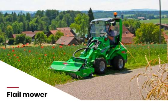
Flail mower is a drum-type cutter, intended for cutting of long grass, scrub, bush and similar vegetation. It will cut up to 20 mm thick tree branches with ease.
