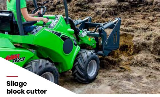
Powerful and robust silage cutters with two hydraulic cylinders. With the silage cutter you can easily cut silage directly from the silo and take it to the cattle. Cutting blades are made of special steel; they cut very efficiently and leave a clean and even surface in the silo. This prevents air getting into silage and warming up. Thanks to the open design of the cutting blade visibility during silage distribution is very good. Lower tines are made of hardened steel.
