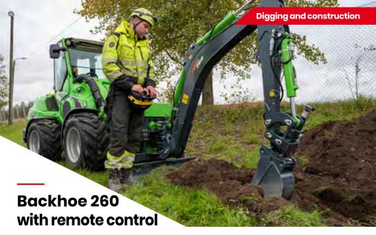
Avant backhoe 260 is now available also with radio remote control (remote control cable is also included). It allows the operator to stand next to the unit when digging and have a perfect, unrestricted field of vision to the work area. This is very useful for utility jobs, cemeteries and similar places where space is limited and exceptionally exact digging with total visibility is necessary.
