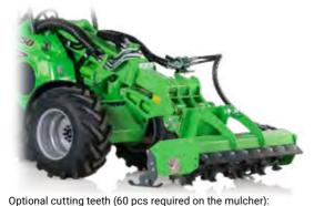
A445791 Rectangular cutter A445804 Conical carbide cutter (standard) A445806 Heavy duty conical cutter A445789 Shearing cutter 66392 & 66393 Cutters (same as on asphalt grinder)
