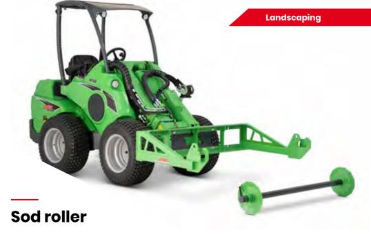
With the sod roller it is easy to lay large sod rolls quickly and conveniently. Sod, also called turf, is the upper layer of soil with grass growing on it and is often harvested in rolls. The roller shaft is designed to slide through the center of the roll; then the roll is picked up by the attachment and the sod can be rolled out.
