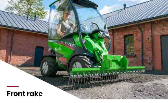
Front rake is an uncomplicated and economical attachment for levelling of sand and gravel driveways, anywhere you want to have a nice looking finish. The spring loaded tines rake and level the ground efficiently. The rake can also be used for loosening and levelling of uneven soils.
