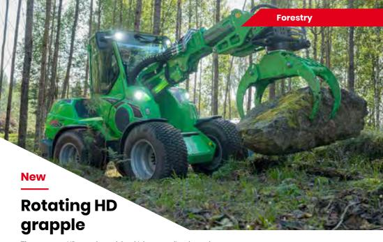
There are two HD grapple models which mount directly on the attachment coupling plate of the loader: one with a hydraulic motor + slewing bearing, allowing unlimited (continuous) rotation in both directions, and one without rotator. They have a different type grapple from the timber grabs. The HD grapple can handle timber as well, but thanks to its sharp claws it can also pick up stones, roots and smaller stumps, as well as remove bushes and other vegetation.
