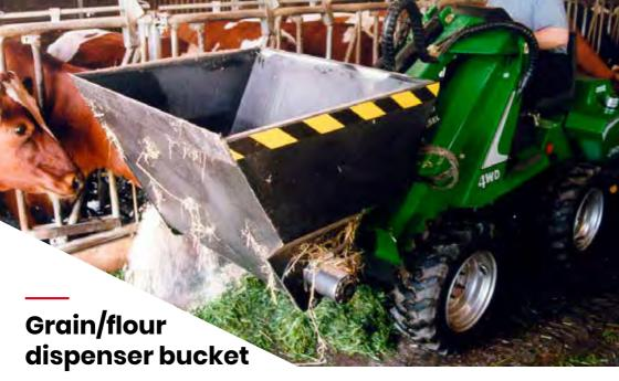
Avant grain dispenser is a 300 l bucket equipped with a hydraulic motor and a Ø 200 mm screw, destined for distribution of flour, crushed grain etc. The bucket is available in two versions: with discharge either to the right side or to the left side.
