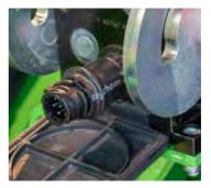
Adapter cable for attachment's multi connector A36679
