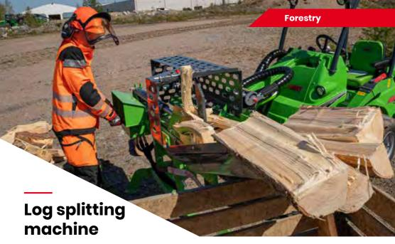
Log splitting machine is the right attachment when you have cut logs and need to make firewood quickly and easily. It is equipped with two-hand operation for increased safety: there are two control levers which have to be activated with both hands before the splitting cylinder will push the log against the splitting wedge. Splitting speed and force can be adjusted if needed.
