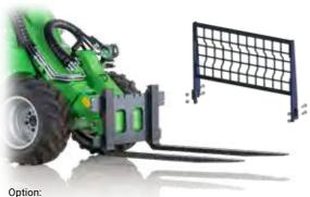
Bolt on back frame A36346 Rotation support, adjustable A441445 (prevents boxes from falling from the pallet fork when rotating & emptying them with the attachment rotator A424406)
