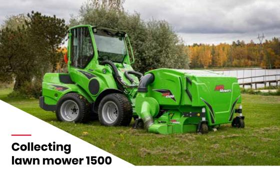
Collecting mower designed for professional use with 1500 mm cutting width and 800 liter collector box. The high suction power makes it also possible to collect tree leaves on lawns. The blades cut the grass, tree leaves etc. to a fine mulch which packs tightly into the collector box.
