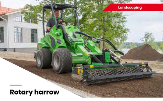
Avant rotary harrow is an excellent leveler for lawn beds, yards, gardens etc. – for places where the ground needs to be perfectly levelled. It harrows only the topsoil and gives a very nice finish for sowing. Required output is lower than that of the rotary hoe, which allows also a higher working speed. Working depth is adjusted with the rear field roller which levels the seeding bed during operation. With the optional seeding unit you are able to make a ready lawn surface on one pass.
