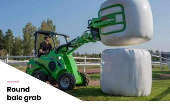
With the round bale grab you can lift and transport wrapped silage bales, hay bales and other round bales without damaging the plastic wrapping or net. Sturdy, yet light construction allows best possible effective load (see the table below).
