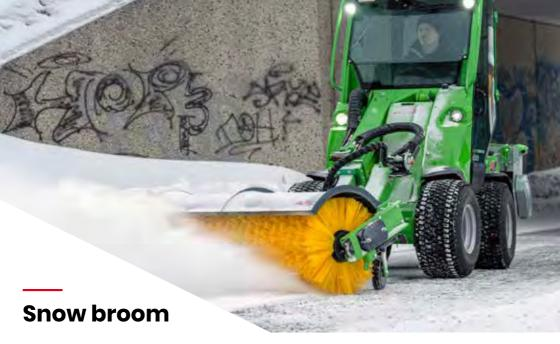
The snow broom is intended for snow removal on sidewalks, parking lots, and more. It features the 550 mm nylon brush and hydraulic motor as the original rotary broom without the vertical floating in the mounting frame. Instead, the brush is supported by two support wheels with solid tires. The height of the support wheels can be adjusted with the nylon spacers on the yoke of the wheel.
