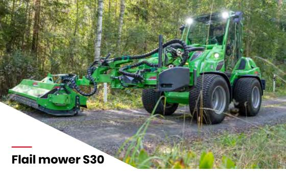
The 1200 mm flail mower with S30 quick attach bracket mounts only on the hydraulic side arm. It cannot be mounted on the attachment coupling plate of the loader or on the S30 mechanical side arm.
