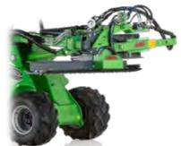
Adapter, for mounting a standard attachment on S30 side arm A460243 The optional Opticontrol® is required on the loader. Extension arm, with manual telescoping 550-950 mm A464146
