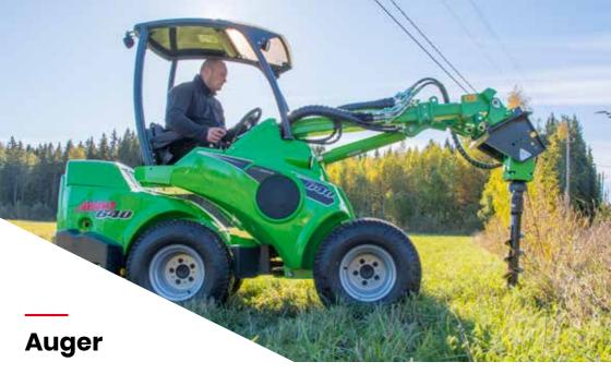
Powerful hydraulic auger with many different auger diameters to suit various tasks, be it post hole boring, tree transplanting etc. Standard drive unit has hydraulic motor and direct drive to the auger. Heavy duty drive unit is equipped with planetary drive to increase torque, needed especially in hard ground conditions or when using large diameter augers.
