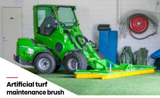
The brush is intended for the daily and weekly maintenance of artificial turf fields. It does not limit or prevent the use of the artificial turf attachment ATA1200, because ATA1200 is intended for monthly maintenance of the field.
