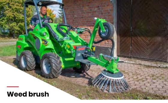
Weed brush is an efficient tool for removal of weeds on all kinds of paved areas etc. It is equipped with a steel brush which can be extended manually and turned in three different positions: to the front, to the right side or to the left side. The weed brush is equipped with a support wheel as standard. It can be lifted and locked up to transport position if needed
