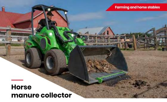
Horse manure collector is a simple and economical way to collect horse manure. It works well on many surfaces (saw dust, horse arenas). Mounts directly on any Avant bucket.
