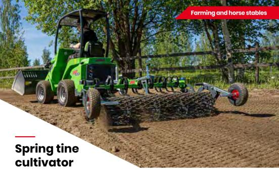
The towable spring tine cultivator with 1500 mm working width is a useful attachment for the maintenance of outdoor horse arenas. for cultivating fields etc. There are 15 spring loaded S tines with replaceable teeth in two rows which cultivate the soil up to 100 mm depth. Working depth can be adjusted by adjusting the height of the rear field roller.
