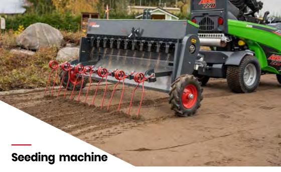
Seeding machine is a professional mechanical surface seeding unit, intended for precise seeding of lawns, different types of (flower) meadows, pastures etc. The rotating feeding roller with 12 nozzles provides accurate and reliable seed sowing, and the seed amount adjustment range is very wide, approx. 50 - 3000 g/100 m2.
