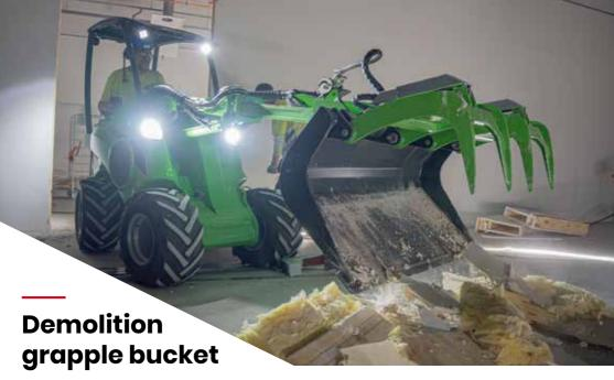
The demolition grapple bucket with two hydraulic grapples **Versatile bucket with two** (1300 mm and 1050 mm) or one (900 mm) are strong and versatile attachment for handling of construction and demolition waste.
