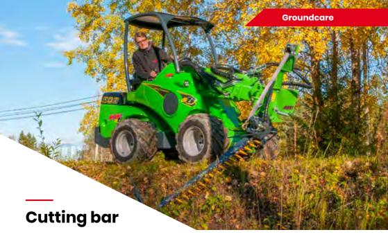
An uncomplicated cutting bar for mowing of hay, grass and trimming of bushes and hedges. Thanks to the side mounting and angle adjustment below ground level mowing of slopes is also possible. Guide plates under the bar support the cutting blades when mowing.
