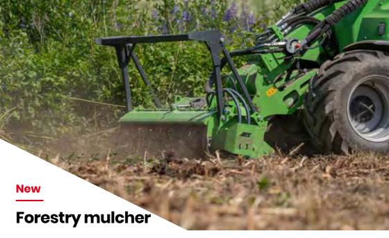
Forestry mulcher is intended for clearing bushes, brushwood and similar vegetation. It can also cut and crush small trees and grind small tree stumps - above ground level. The mulcher features direct hydraulic drive: a hydraulic motor is mounted on the rotor Opinect hydraulic drive, rotor which is equipped with crushing and mulching type carbide teeth.
