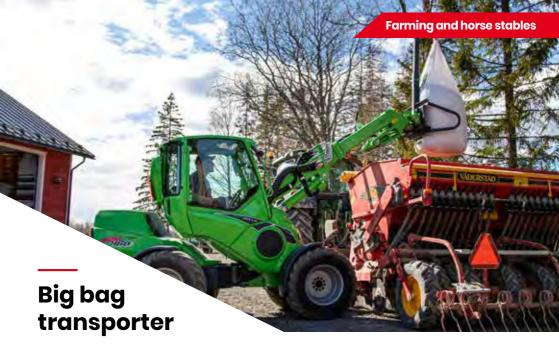
With the big bag transporter you can lift and transport big bags safely and securely. This simple attachment makes loading of fertilizer or stacking big bags as easy as it can get.
