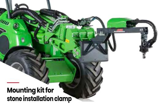
For professional paving, a hydraulic stone installation clamp is OCE marked "plug and play" a fast and easy way to lay paving stones. The installation clamp takes a whole layer of stones from the pallet, which then can be lifted directly to the area to be paved. Avant is an ideal machine for this job thanks to the articulated chassis which allows driving on the paved surfaces without damaging them, and thanks to the rigid articulation joint Avant loader is very stable also in paving jobs.
