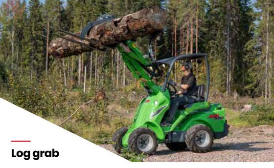
The Avant log grab mounts on Avant pallet fork. With the log grab you can lift and transport single logs or smaller timber bundles. The grab is equipped with a powerful hydraulic cylinder and can therefore also lift bigger stones, as well as branches, fence poles and similar objects.
