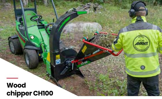
Wood chipper CH100 is a compact and robust disc chipper which works also on Avant 200 series 2 and 400 series. With it you can chip branches and small trees up to 100 mm diameter - an ideal tool for chipping wood in smaller scale. Two knives and an anvil take care of chipping and feeding. Wood feeding is manual.
