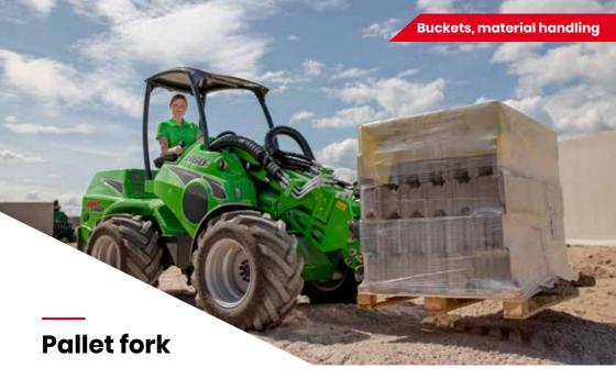
Avant pallet fork is the right attachment for lifting and handling of different types of materials on pallets. Fork width can easily be adjusted thanks to the quick lock mechanism. The forks are made of high tensile forged steel and designed in accordance with the ISO2330 standard.
