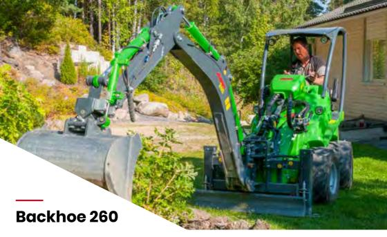
Backhoe 260 has many improved features: Boom swing happens with two hydraulic cylinders, instead of the single cylinder and chain drive in the old models. The new system gives more exact boom movements when swinging and requires less service. Swing angle is 170 degrees. Backhoe 260 is equipped with hydraulic outriggers as standard. The operator can easily adjust the outriggers with
