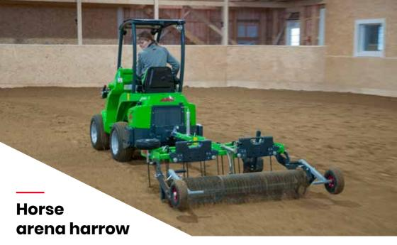
The horse arena harrow is intended for levelling and loosening of horse arena riding surfaces. The harrow has two spring loaded tine rows which loosen the surface, a leveller that makes the surface completely even and a tilling roller that compacts the ground and leaves a finished surface perfectly suited for horse's hoof. The harrow doesn't damage the lower levels (understructure) of the riding surface.
