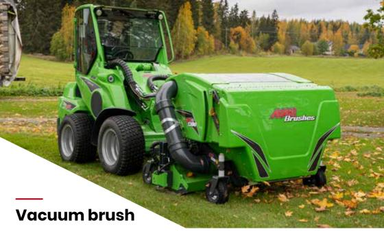
The vacuum brush is intended mainly for collecting of tree leaves in parks, lawns, yards etc. The powerful vacuum unit sucks the waste first into the vacuum on the bottom of the collector box and then into the box, compacting everything into a tight package. The mouthpiece on the vacuum is equipped with a 1300 mm wide rotary brush which loosens also more compacted and wet leaves and waste. Brush rotation speed can be adjusted steplessly.
