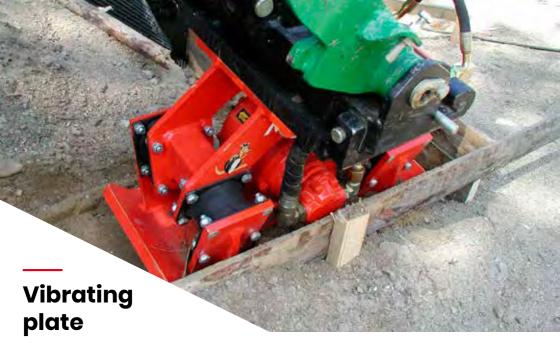
Vibrating plate is designed for earth compacting and is easy to Efficient compacting also in places attach to an Avant. Compacting is easy and safe with the vibrating plate connected to Avant's quick attach plate - the operator is not exposed to vibrations or excessive noise.
