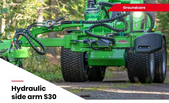
The hydraulic side arm with S30 quick attach system can be equipped with attachments with the corresponding S30 quick attach bracket.
