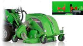
Option: Mounting plate for 200 series, increases tipping angle by 30° A37315
