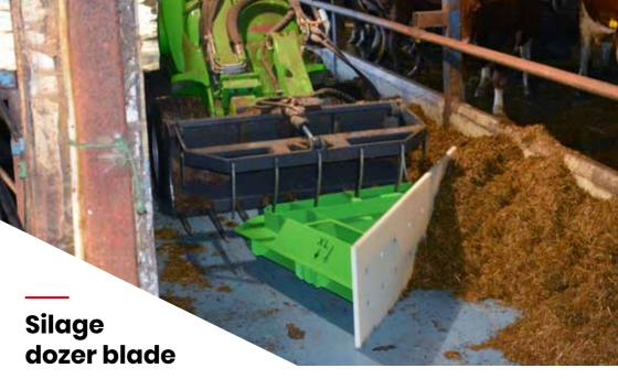
Intended for moving uneaten silage back to the cattle on the feeding table. Mounts on the normal or XL silage grab simply by closing the upper grapple on the dozer blade. The blade can be grabbed with the silage grab from two sides which means that it can move the silage both to the right or to the left. Equipped with a durable nylon blade.
