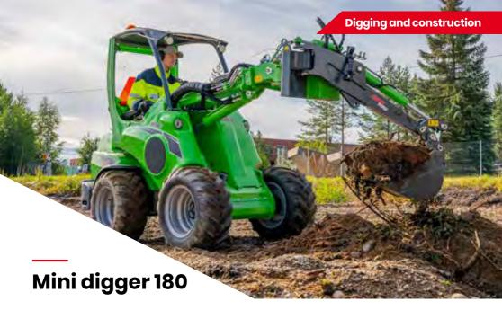
Mini digger 180 features hydraulic boom swing: the boom can be turned 60° to the right or to the left from centerline. This makes the mini digger even more versatile than before:
