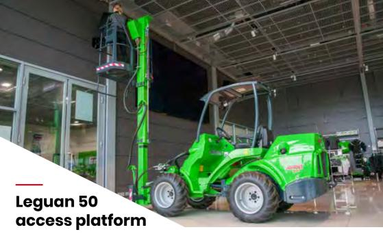
Avant and its daughter company Leguan Lifts have joined their forces and created an acces platform which is mounted directly into Avant loaders quick attach plate. The result is an inexpensive, handy and easy to use acces platform. With the help of this lift Avant's versatility is further increased on the job sites.
