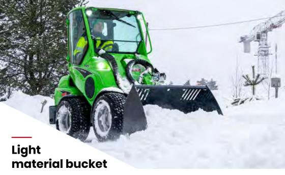
Light material buckets are intended for handling of e.g. snow, saw dust, manure, wood chips and other light materials.
