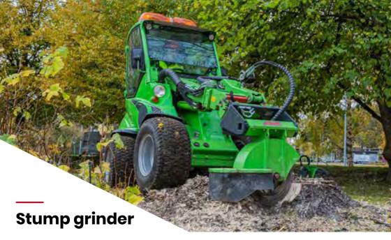
Avant stump grinder is an efficient and easy to operate tree stump remover. The cutting disc is mounted crosswise in relation to the loader, which means it throws the wood waste to the right side the waste doesn't fly on the operator or the loader. In addition, the stump grinder is equipped with a protective rubber cover which prevents the wood from flying around.
