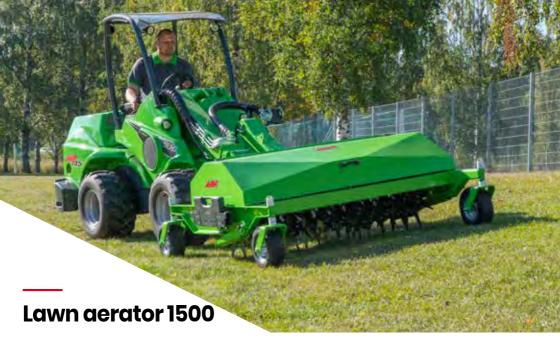
Lawn aerator is designed to create holes in the lawn surface which encourages free movement of soil. This helps to improve the circulation of air in the soil which is vital for a healthy lawn. Avant aerator is completely mechanical - when driving forward with the loader the knife type tines on the aerator shaft turn and make holes in the lawn.
