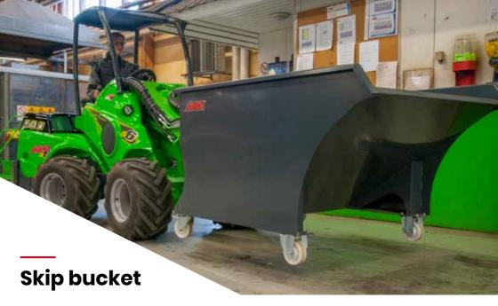
The skip buckets are more like skip containers, but can be transported and emptied easily with Avant. The bucket can be equipped with castor wheels as an option. With them the bucket can be moved and filled by hand effortlessly e.g. in horse stables, on factory floors and similar tight situations where driving with the loader is not necessary or possible. A full bucket can then be taken away and emptied with Avant.
