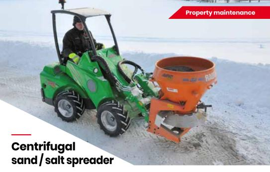
Centrifugal sand or salt spreader is the right choice for winter maintenance of large areas. Both the spreading area (2 to 6 meters) and the spreading amount can be adjusted either manually (standard) from the side of the spreader - or electrically from the driver's seat (option). This guarantees fast and efficient spreading.
